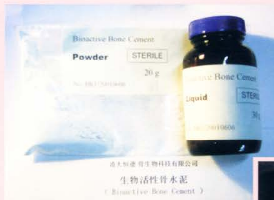
Fig 1 Sample of injectable bioactive bone cement consisting of strontium-containing hydroxyapatite (Sr-HA) (含鐿經基磷灰石) filler and D-GMA resin (縮水甘油樹脂) — developed from the biomaterials laboratory of the Department.
