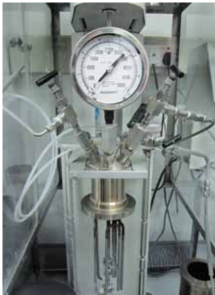
Parr 4547 large scale hydrothermal reactor for all kinds of biomaterials
