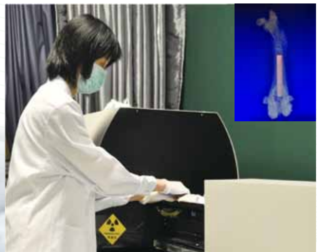
Above: A post-graduate student using a specialised Micro-CT scanner for determining bone mass in small laboratory animals .
